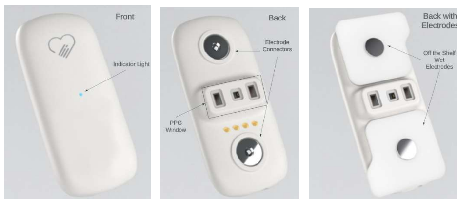
Figure 1. CardioTag wearable device showing front (left), back (middle), and back with electrodes connected to the snaps (right) views. (*note: actual colors may vary)
